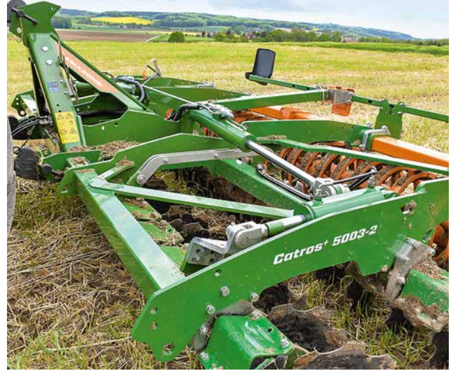
△ A linkage connects the two disc gangs. The working depth is set independently of the trailing press.
